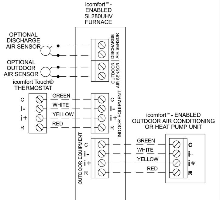
**NOTE** - On communicating systems, extra wires must terminate on the "C" icomfort™ terminal strip (RSBus). Use an additional wire and come off "C" terminal and wire nut all the extra wires together. Termination on the outdoor control must match the indoor control.
