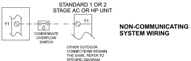
**NON-COMMUNICATING SYSTEM WIRING**
