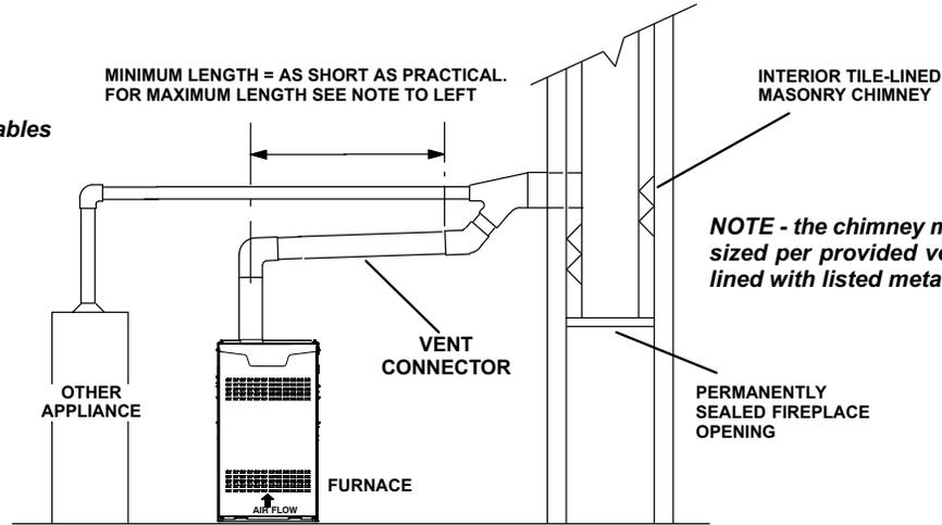
**NOTE - the chimney must be properly sized per provided venting tables or lined with listed metal lining system.**
